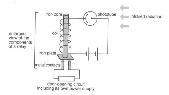
When a current flows in the phototube circuit there is a magnetic field in the coil in the relay.
