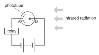
When infrared radiation shines on plate A, electrons flow in the circuit.
