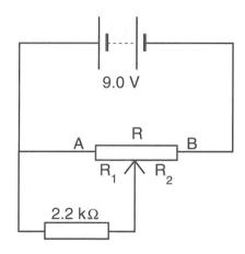
The potentiometer consists of a single resistor of resistance R which can be divided into two resistors of resistances  $R_1$  and  $R_2$  in series, by changing the position of a sliding connector. The total resistance R stays constant and is always the sum  $R_1 + R_2$ , of the values of the two resistances. The total resistance R of the pot is 4.7 k $\Omega$  (4700  $\Omega$ ).
