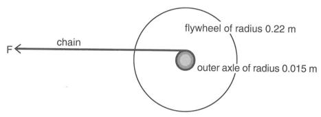
Pulling on the chain causes the flywheel to rotate without any slipping occurring between the axle and the chain.
